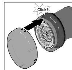
Always attach the protective cap when the device is not in use. You should hear and feel it click into place.
